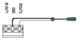
Figure 14: IR Emitter Wiring
